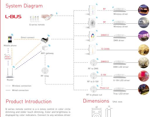
within effective distance and keep the effect in sync. Working with F4-5A, F5-DMX-4A and touch panel, etc.
